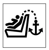
To assist you in locating the top tether anchors, the top tether anchor symbol is located on the trim cover.
